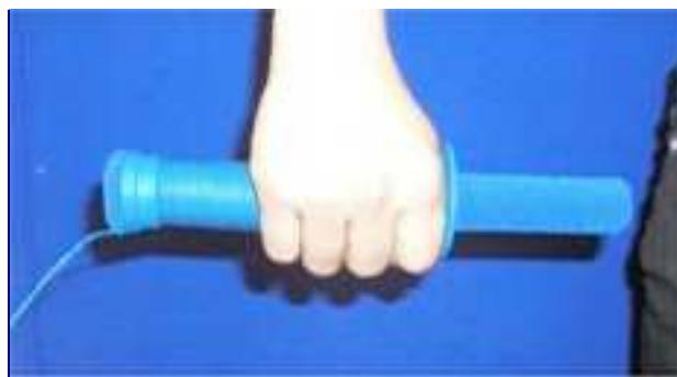
Figure 3-4: The handles have a button and cable connected allowing the subject to initiate the image capture.
